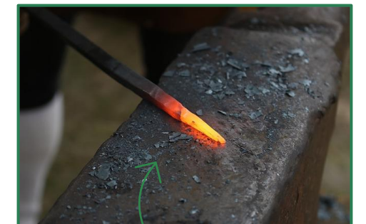
The hotter the iron, the brighter and whiter it glows!
